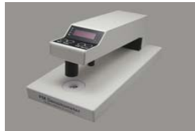
Figure 1: The novel compact densitometer especially designed for a convenient measure of optical absorption of standard D-Squame® strippings (Ø 22mm).
